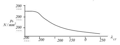
Fig. 18 Bending strength for rolled sections of design strength 240  $N/mm^2$
