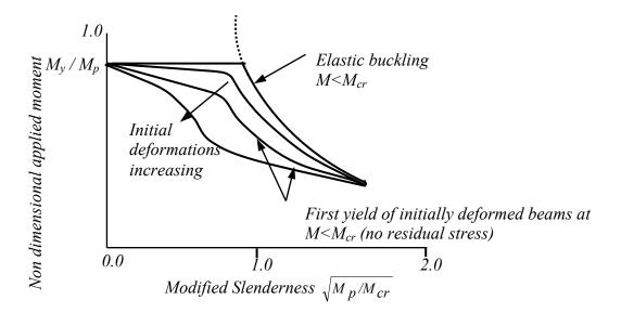
Fig. 16 Beam failure curve
