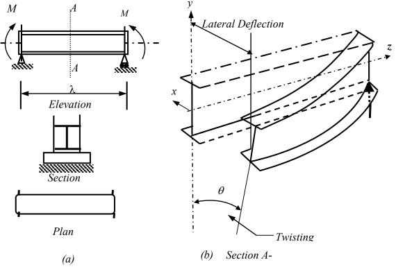
Fig. 5(a) Original beam (b) laterally buckled beam
