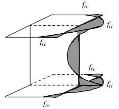
Fig. 15 Residual stresses in I beams
