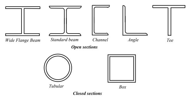
Fig. 4 Open and closed sections
