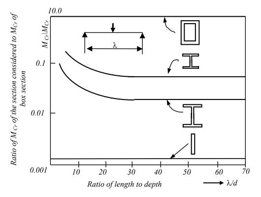
Fig. 12 Effect of type of cross section
