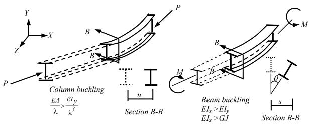
Fig. 3 Similarity of column buckling and beam buckling
