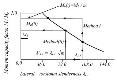
Fig. 10 Moment capacity of beams
