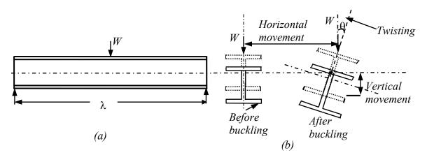
Fig. 2(a) Long span beam, (b) Laterally deflected shape of the beam
