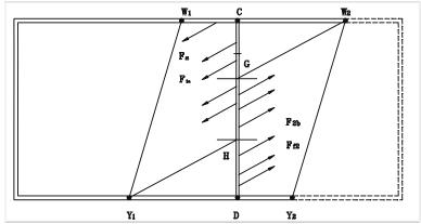
Fig. 10 Force imposed on transverse stiffeners by tension field
