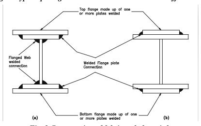
Fig. 2 Cross-section of fabricated plate girders
