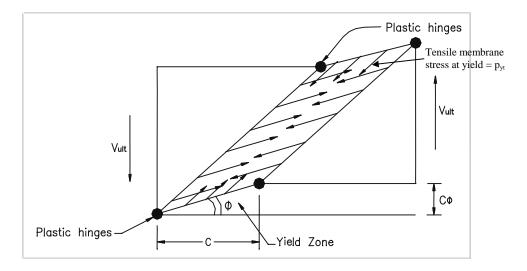
Fig. 6 Collapse of the panel
