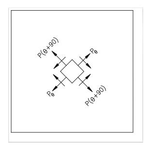
Fig. 4 Post buckled behaviour
