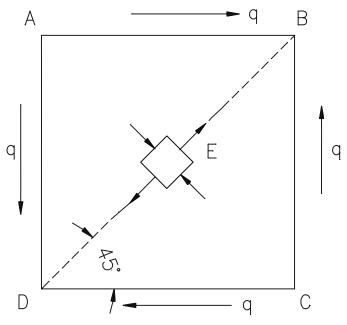
Fig. 3 Unbuckled shear panel
