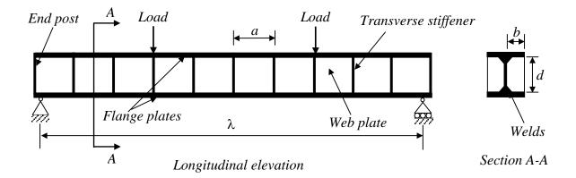
Fig. 1 A typical Plate Girder
