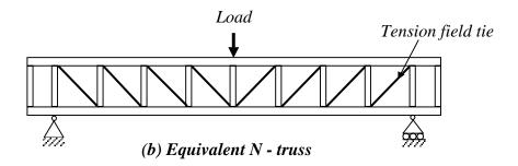
Fig. (3) Tension field action and the equivalent N - truss
