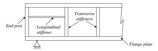
Fig. 2 End panel strengthened by longitudinal stiffener 1.3 Recommended proportion of flanges
