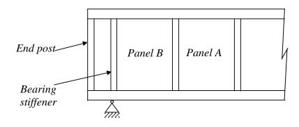
(d) End panel designed using tension field strengthened by additional stiffener (Double stiffener)
