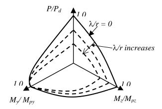
Fig. 8 beam-columns under Biaxial Bending
