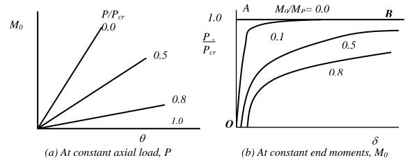
Fig. 5 Elastic Behaviour of Beam-Columns
