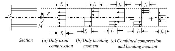
Fig. 2 Stresses in Short Beam-Columns
