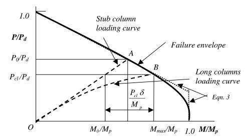
Fig. 3 Beam-Column Failure Envelope
