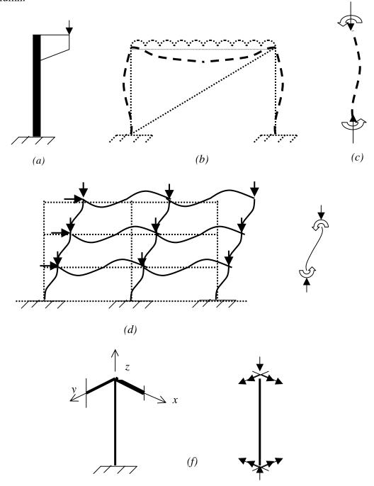
Fig. 1 Beam-Columns in Frames
