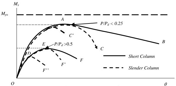
Fig. 7 Beam-column Moment Rotation Behaviour
