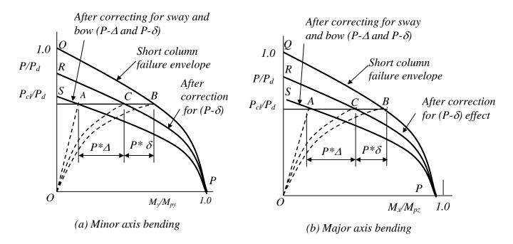
Fig. 6 Uniaxial Bending of Slender Beam-Columns
