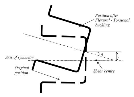
Fig. 3 Column displacements during Flexural - Torsional buckling
